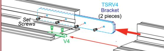
3. Use Set Screws to secure extrusions.
