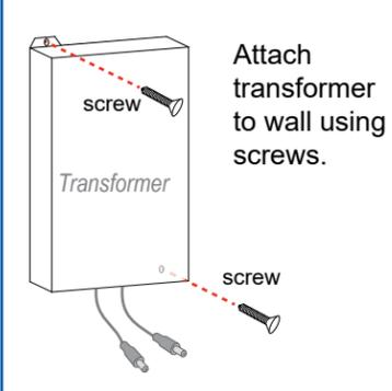
Attach transformer to wall using screws.
